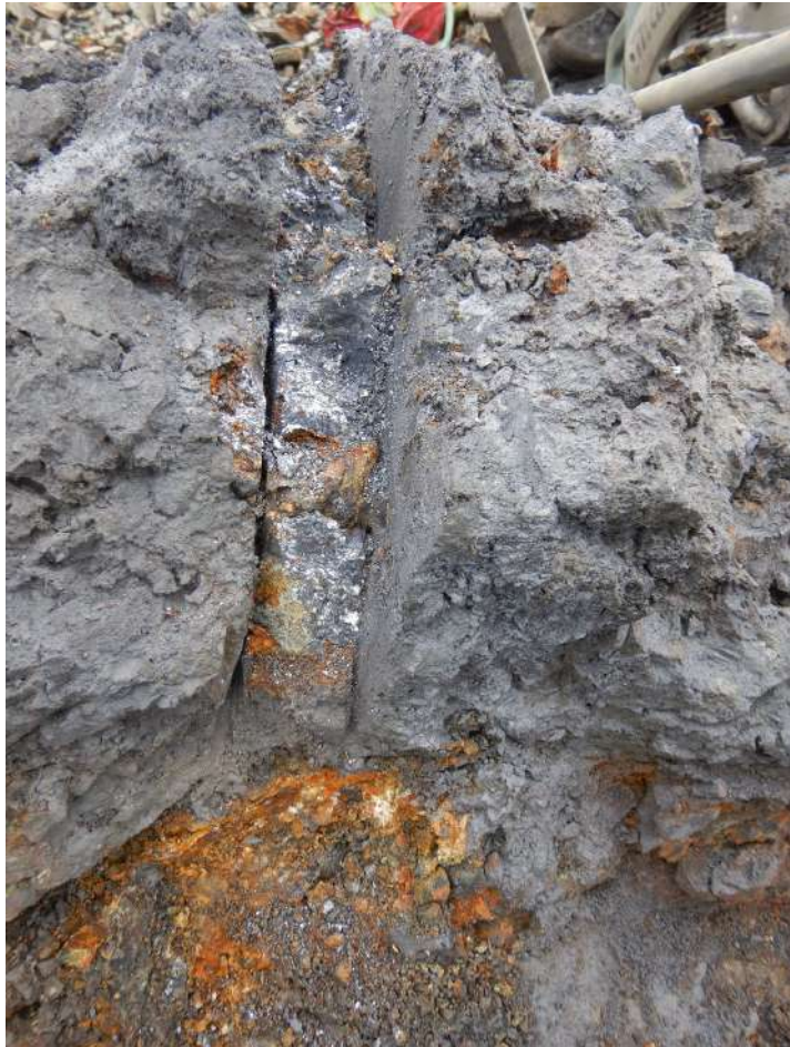
P2 Vein channel sample 1775 g/t Ag, 48.8% Pb and 13.4% Zn over 1.2 m
