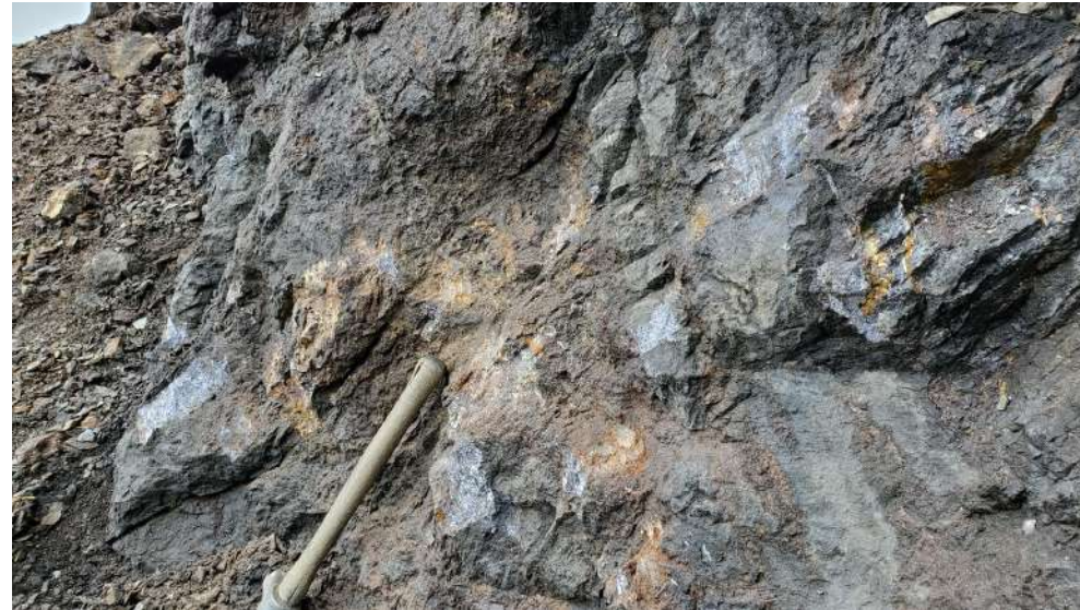
P2 Vein chip sample 4300 g/t Ag, 46.4% Pb and 22% Zn over 1 m.
