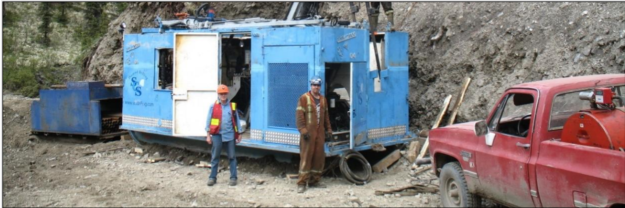
Figure 10-2: HTM-2500 Skid-Mounted Diamond Drill Rig at Casket Creek
